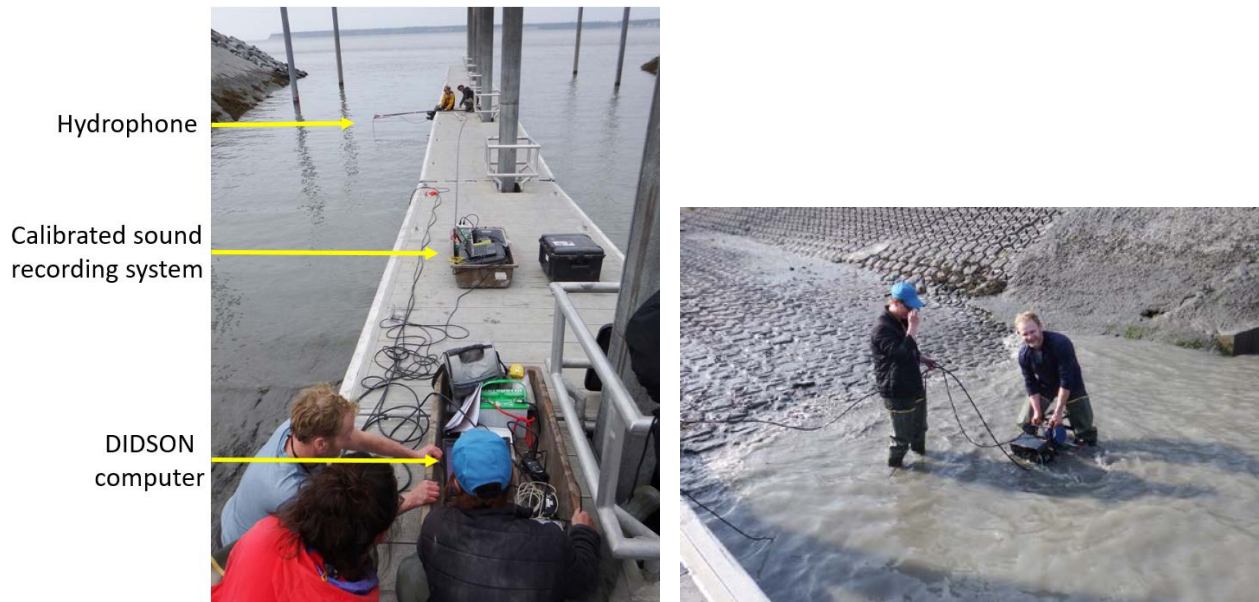
Figure 6: Left - Calibration procedure at the small boat launch ramp in Anchorage, AK. Hydrophone is placed on axis guided by the DIDSON field of view at different distances. Right - the DIDSON transducer and underwater speaker system, attached to their tripod plate, are placed at the end of the concrete ramp at low tide, with the center axis of the field of projection parallel to the dock.
