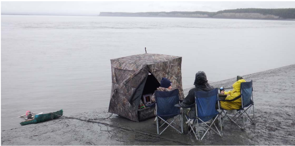
Figure 4: Pop-up hunting blind protecting the laptop and sound system. The sled is semi submerged on the left placing the DIDSON transducer and speaker underwater.
