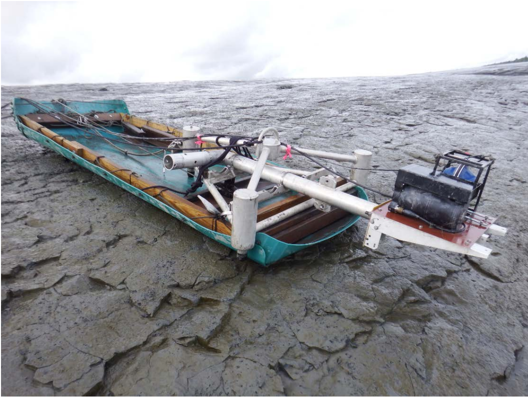
Figure 2: Custom built sled and adjustable tripod to deploy the DIDSON and underwater speaker system in the beach, allowing adjustments while submerged. The sled was pulled or lowered every few minutes to follow the tide.
